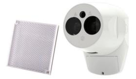
The FRAY-ONE-EN is an easy to mount and costeffective linear beam detector. It covers distances between 5 m and 120 m. A reflective prism allows for the accurate detection of smoke particles within the given distance range.
